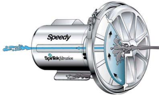
Figure 13: Flow Path of Rotary Filter
