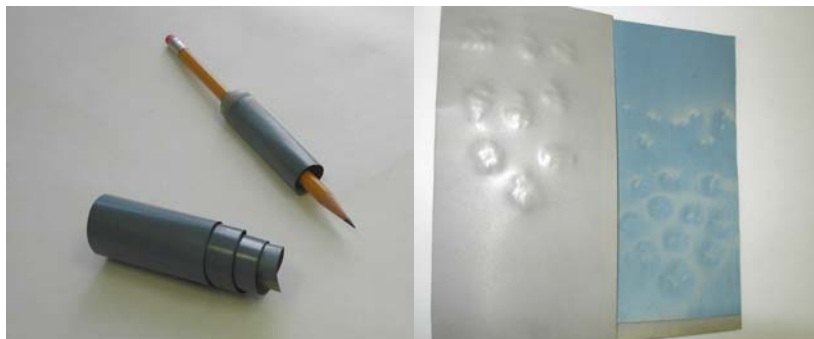
Figure 2: Alloy Filter rolled around a pencil and struck with a hammer
